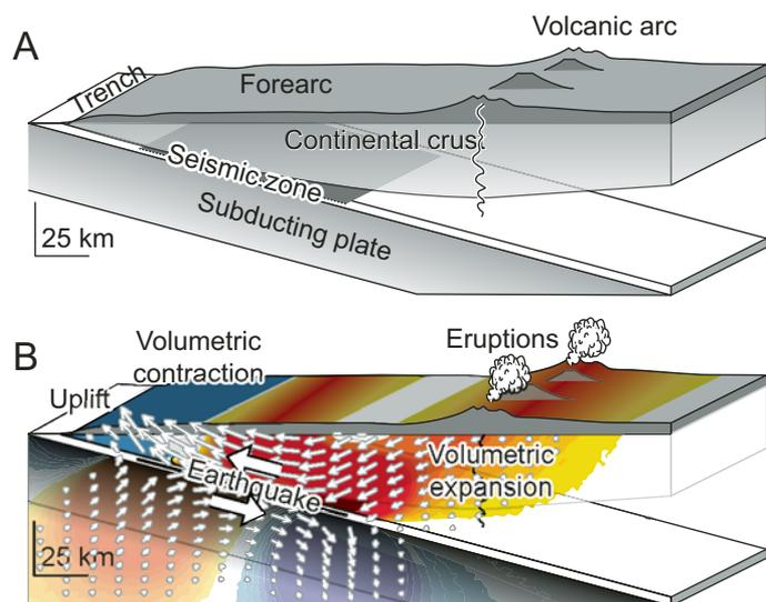
**Figure 2. A: Schematic cross sections of subduction zone. B: Displacement field (arrows) and volumetric deformation (red colors for volumetric expansion, blue colors for volumetric contraction) associated with megathrust earthquake. Volcanic system undergoes volumetric expansion by earthquake.**
