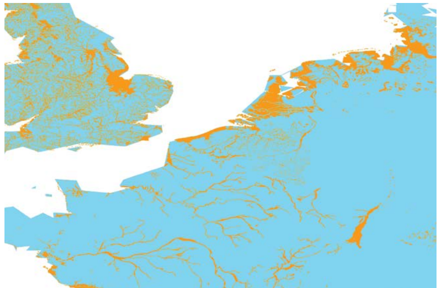
Figure 2. Example of coastal and inland areas with Holocene sediments, including clay and peat (white areas), in the central part of Europe. These areas, in most cases in deltas and in river basins, are prone to subsidence. (Source: http://www.onegeology-europe.org/ ).
