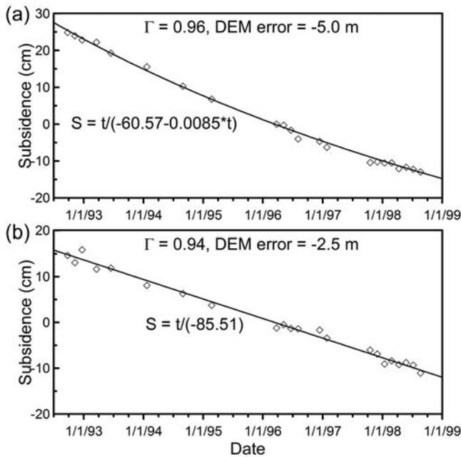
**Figure 2.** Temporal behaviors of the subsidence measured at two selected (a) point A and (b) point B in Figure 1. Hyperbolic model solutions for deformation estimated from PSI method are also displayed. Note that the model parameter  $v_b$  (see equation (2)) at the point B is zero, consequently the model solution is identical with the linear model. Temporal coherence  $\Gamma$  and DEM error estimated during PSI processing are presented in the plots.
