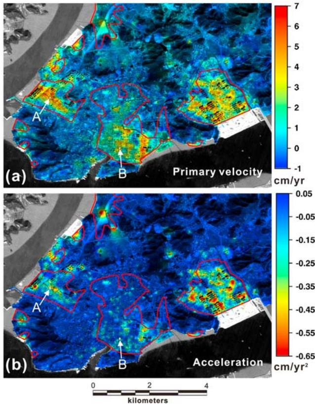
**Figure 1.** Subsidence map of Mokpo city derived by means of JERS-1 PS analysis using hyperbolic model. (a) Primary velocity and (b) acceleration term at the PSs calculated from equation (4). Both maps were calculated on regular spatial grid by means of Kriging interpolation. Background image is optical satellite image, and red polygon represents the main reclaimed area. The temporal evolution of the deformation at two PSs marked by A and B are shown in Figure 2.
