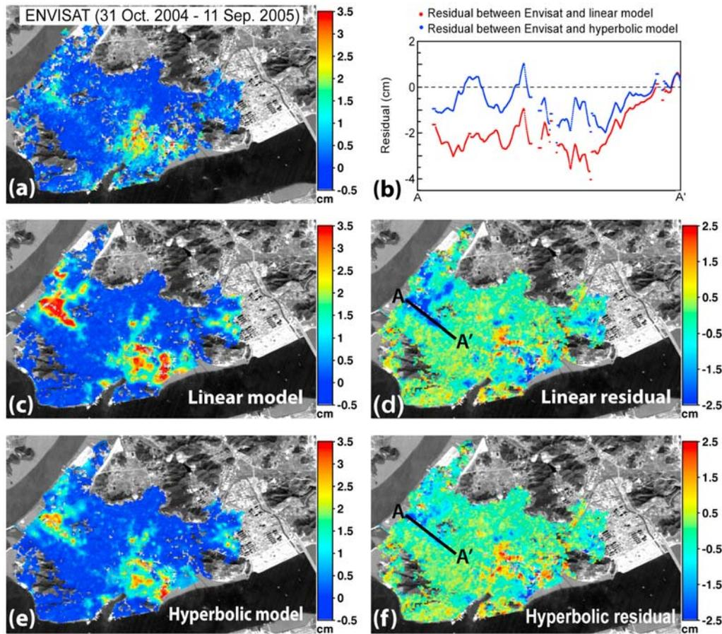
**Figure 3.** Comparison between linear model and hyperbolic model using ENVISAT measurement. (a) Subsidence derived from ENVISAT InSAR pair (31 Oct. 2004 and 11 Sep. 2005), (b) two model's residual deformation at profile A-A', (c and d) linear model and residual for the subsidence during the ENVISAT observation, (e and f) hyperbolic model subsidence and residual. The subsidence from 2004–2005 is better described by a hyperbolic model.
