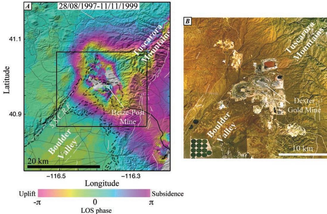
**Figure 3.** Bedrock subsidence (a) 2 years interferogram of the bedrock subsidence in Tuscarora mountain over shaded relief of topography. Southern Sheep Creek Range Fault (S.S.C.R.F.). Faults (white lines), main roads (grey lines), bedrock-sediment limit (dashed black line). (b) Landsat image of the Dexter Mine complex.
