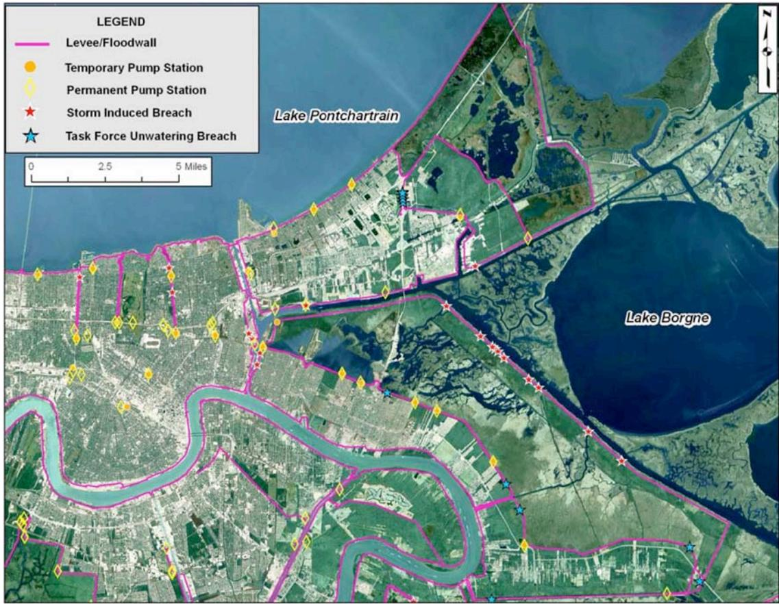
Figure S4. Map of breached levees in St Bernard Parish<sup>24</sup>. Note breached levees along MRGO, corresponding to high subsidence rates (Figure 1, inset).
